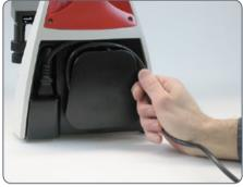
Proper storage of accessories in the appropriate positions is important to keep them safe from loss or damage. There are storage places for the objective centering tools and for two compensators in the rear of the Analyzer/Bertrand Lens module.
